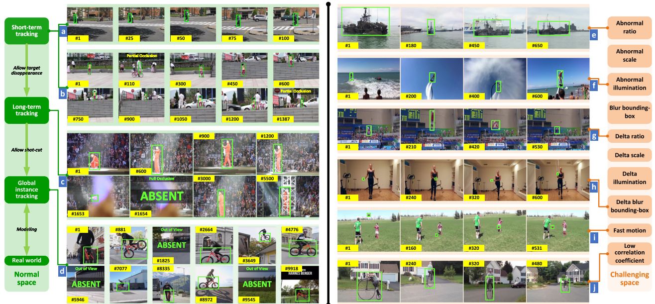
Fig. 4 Examples of normal space E_n and challenging space E_c . Sequences in E_n are selected from existing datasets, while sequences in E_c are obtained based on space construction rules
